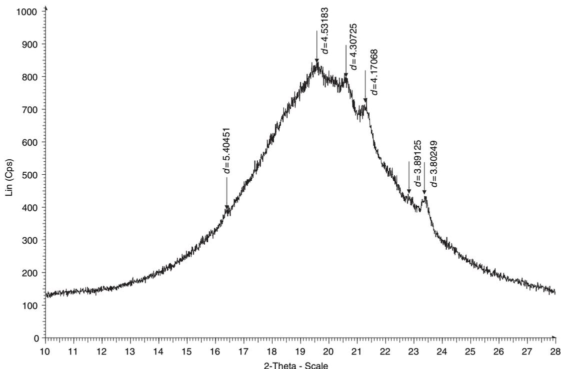
FIG. 4—Diffractogram of fat sample.
